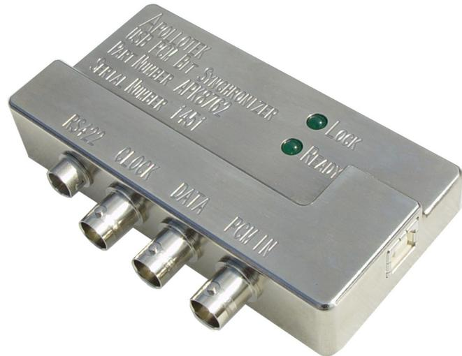
The Apollotek APK8762 Bit Synchroniser is part of the ApolloDas range of USB products which are designed for PCM Flight Test Instrumentation system checkout and test applications. The unit is supplied in an aerospace grade aluminium housing machined from solid which is rugged enough to be installed in an aircraft.
